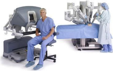
Figure 1: Da Vinci System. Surgeon's console (left) and nurse on operating table next to robot arms.
